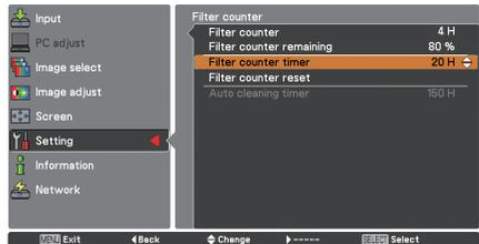
Press the SELECT button to select Filter counter timer and use the Point ▲▼ buttons to set the timer. Select from (Off/ 10H/ 15H/ 20) depending on the use environment.
