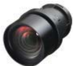
AH-24721 • Power, Fixed FL: 0.51" (13.05 mm) f:2.0 On Axis T/W: 0.8:1
