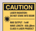
This warning is required by the U.S. FDA and pertains to the laser pointer in the wireless remote control of this projector.
