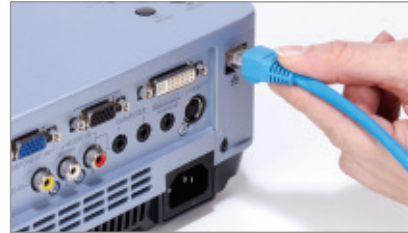
Built-in RJ-45 LAN port.
