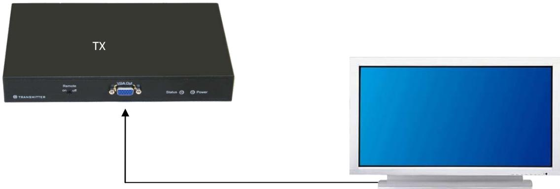
Lastly, power up the unit by plugging in its power adapter. The POWER LED should be RED, and the STATUS LED should be GREEN.
