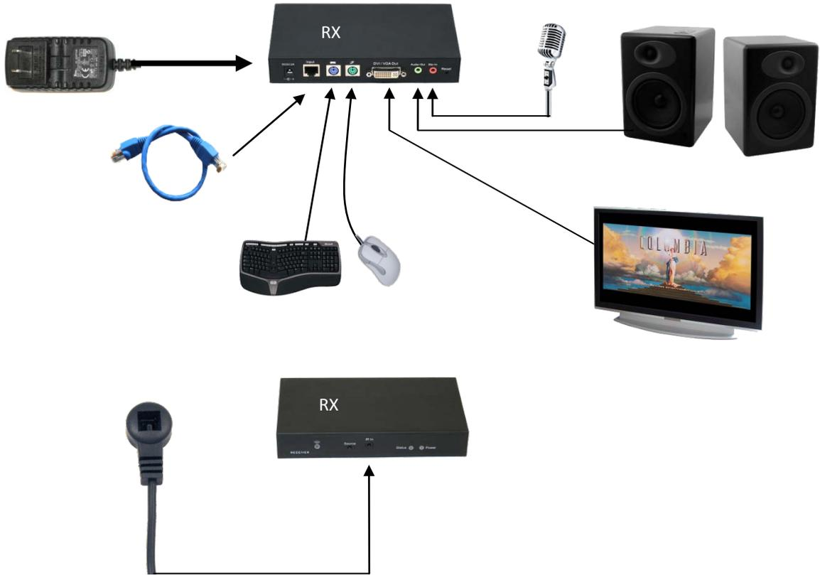
The included all-in-one cable can be used to extend the devices if the RX is in an inaccessible location.
