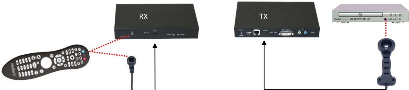
Simply plug in the PS/2 devices into their respective ports on the transmitter, then power up the receiver. On the transmitter side, use the included USB cable to connect the transmitter's USB port to an unused USB port on the computer. Your computer may prompt you that it has detected new hardware, so just follow the prompts to complete the installation process.
