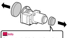
If you try to attach the lens to the projector without removing this cap, the optional lens attachment part can be damaged.
