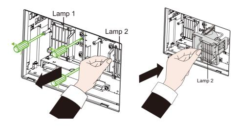
4. Insert the lamp, tighten the three screws and make sure the lamp is firmly secured to prevent the lamp from shaking or poor contact.
