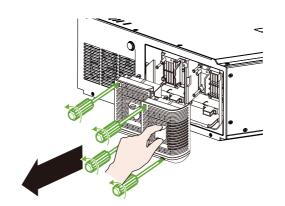
3. Loosen the screws and pull the lamp module out.
