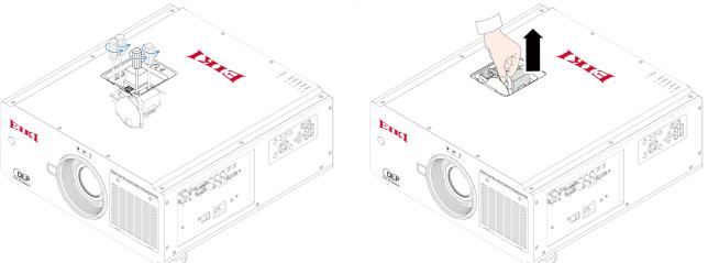
3. Place the color wheel and tighten the four screws.
