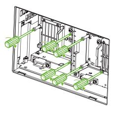
5. Install the fan unit and tighten the two screws on it.
