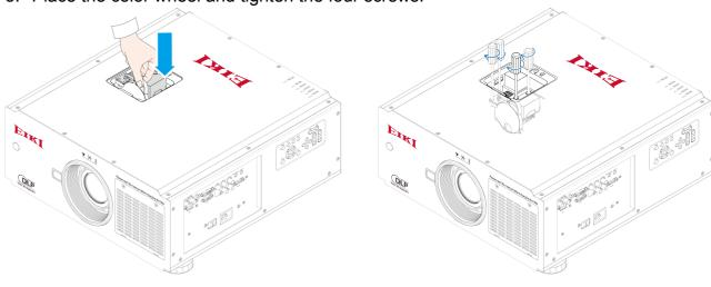
4. Place the color wheel cover and tighten the screw.
