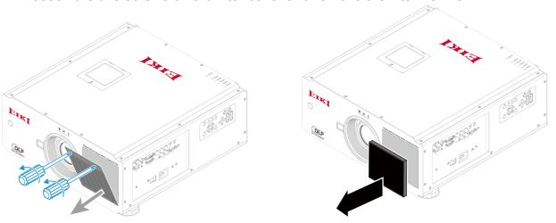
2. Place a new filter and install the filter cover. Tighten the two screws on the filter cover.
