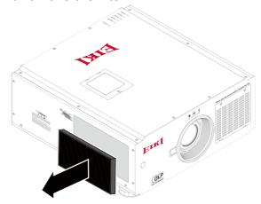
2. Place a new filter and install the filter cover. Tighten the two screws on the filter cover.
