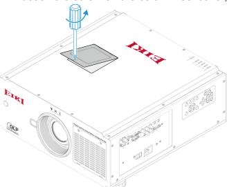
2. Loosen the four screws on the color wheel, and remove the color wheel.
