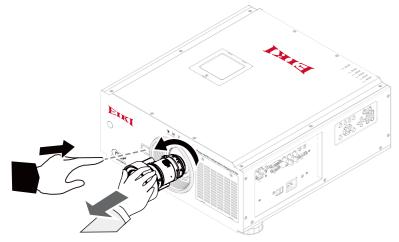
2. Insert the lens and ensure the lens touches the lens holder. Align the "\\_" symbol on the lens label with the "\\_" symbol on the top of the body (align to the center of the lens hole).
