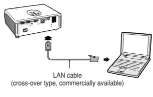
A LAN cable being connected to the network
