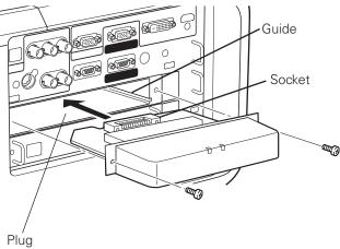
Figure shows HD DATA WIRELESS Receiver Board
