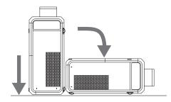
When moving the projector by one person, grip handles and carry it with lens side up. Then, lay it down on the correct position.
