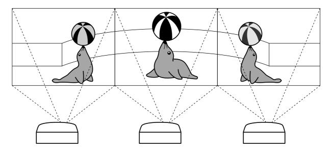
To create the wide video wall with three projectors lining up in single file from left to right (as shown above), select "3 X 1" on "Division", select a position for each projector, and then input the image which width is compressed at 1/3 (as shown below).
