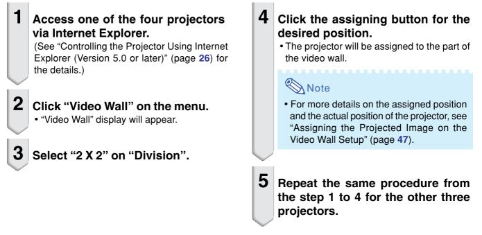
That completes the video wall setup. When the same image signal is input to all the projectors, the video wall projection starts.
