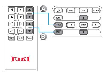
Use the Keystone H buttons (on the remote control) to adjust the keystone horizontally and make a squarer image. Use the Keystone V buttons (on the remote control) to adjust keystone vertically and make a squarer image.
