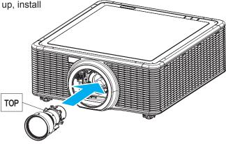
$\boldsymbol{5}.$  Rotate the lens clockwise to lock the lens in place.
