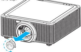
**3.** Remove both lens caps (front and back) on the lens.
