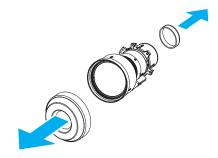
**4.** With the label "TOP" on the lens assembly facing up, install the assembly into the lens mount.
