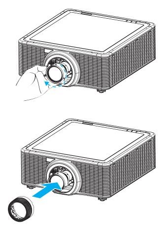
**6.** Firmly install the lens cover onto the lens.
