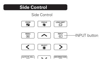
The input source changes each time you press the INPUT button on the side control as follows: Input  $1\rightarrow$ Input  $2\rightarrow$  ...
