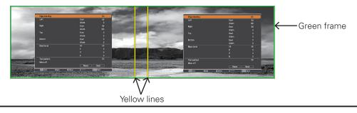
5 Set Test pattern to On to display a 50 % white image. The overlap area will be brighter than the non-overlapping area. Adjust the Black level in the Edge blending dialog box to increase the brightness of the non-overlapping area so that the unevenness is reduced.
