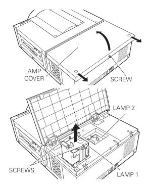
Make sure which number of lamp needs to be replaced on Lamp Status Display.
