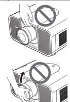
Do not hold the lens and the peripheral part.
