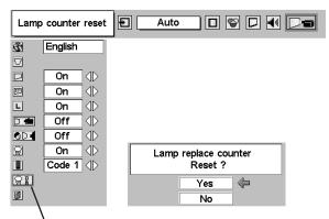
Move the pointer to Lamp counter reset and then press SELECT button. The message "Lamp replace counter reset?" is displayed.
