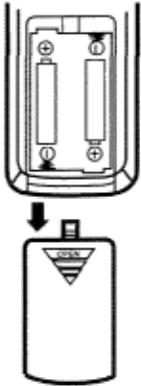
**2** Slide the batteries into the compartment.
