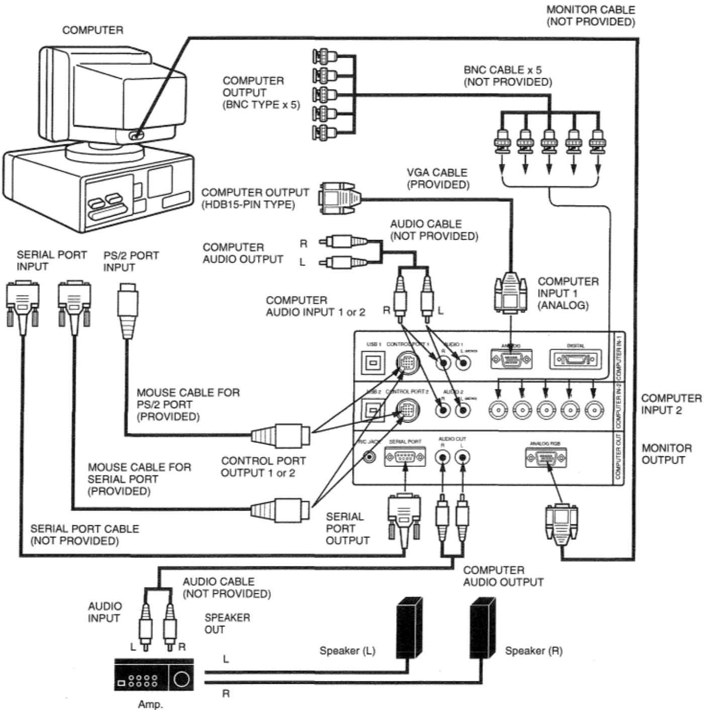
**NOTE:** When connecting the cable, the power cords of both the projector and the external equipment should be disconnected from AC outlet. Turn the projector and peripheral equipment on before the computer is switched on.
