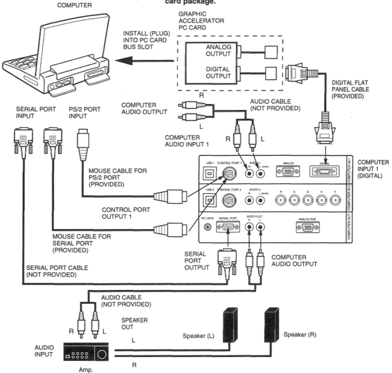
NOTE: When connecting the cable, the power cords of both the projector and the external equipment should be disconnected from AC outlet. Turn the projector and peripheral equipment on before the computer is switched on.
