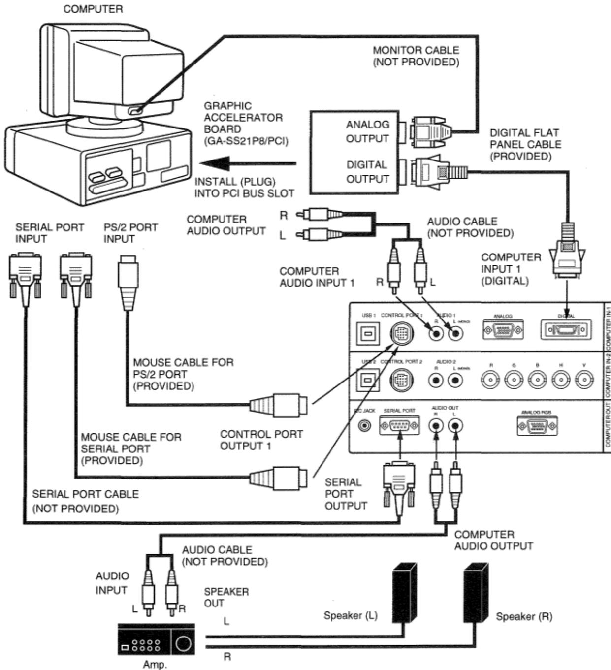
**NOTE:** When connecting the cable, the power cords of both the projector and the external equipment should be disconnected from AC outlet. Turn the projector and peripheral equipment on before the computer is switched on.
