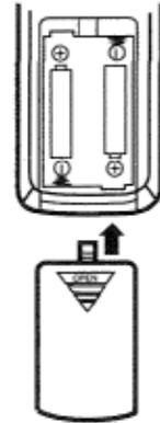
The remote control unit can be used as wireless or wired remote control.
