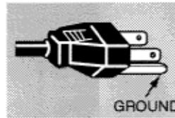
This projector is equipped with a grounding type AC line plug. Should you be unable to insert the plug into the outlet, contact your electrician. Do not defeat the safety purpose of this grounding type plug.
