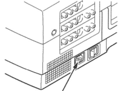
Connect the AC power supply cord (supplied) to the projector. The socket-outlet must be near this equipment and must be easily accessible.
