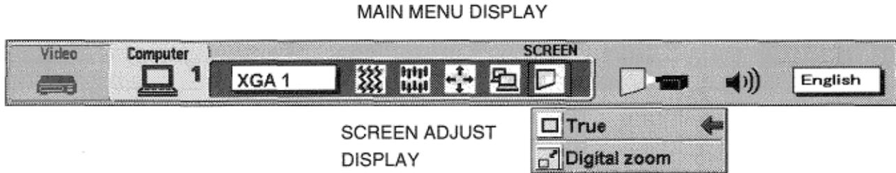
4. To adjust the image size or pan the image, move the arrow to Digital zoom by pressing POINT UP/DOWN BUTTON(s) and then press SELECT (REAR CLICK) BUTTON. MAIN MENU DISPLAY and SCREEN ADJUST DISPLAY will disappear. The "D.zoom" and the magnifying-glass icon is displayed to indicate Digital zoom mode.
