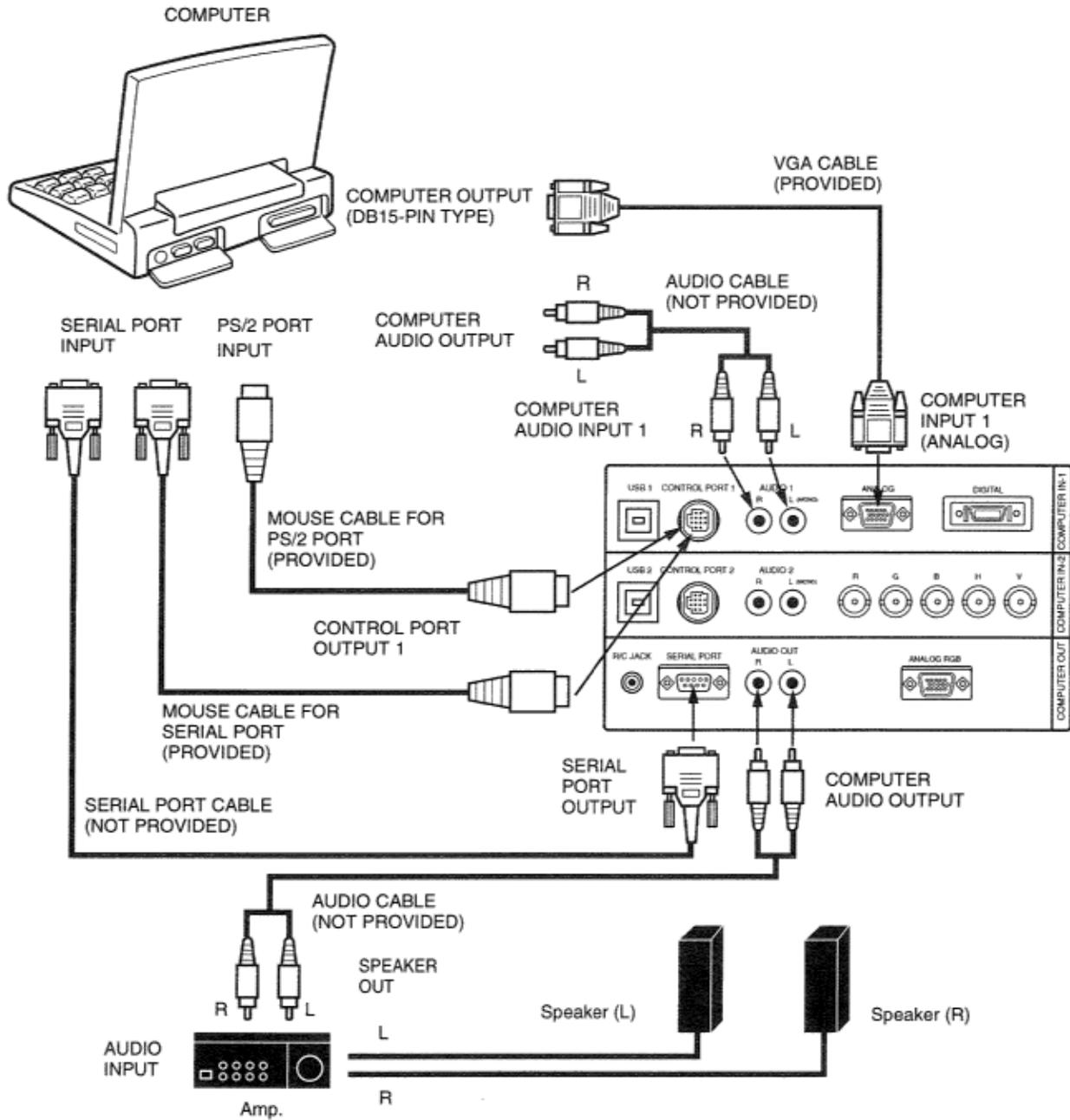
**NOTE:** When connecting the cable, the power cords of both the projector and the external equipment should be disconnected from AC outlet. Turn the projector and peripheral equipment on before the computer is switched on.
