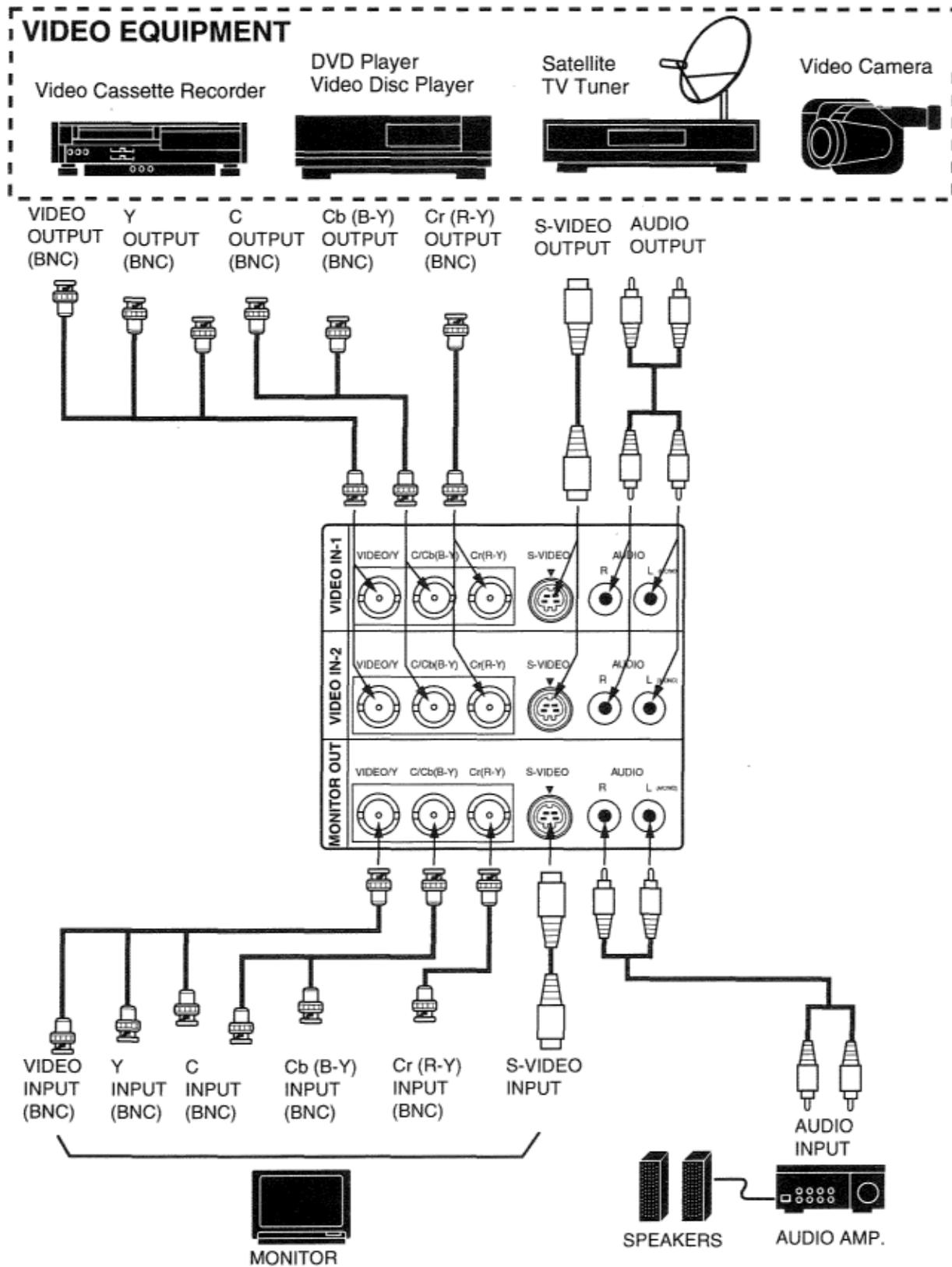
NOTE: When connecting the cable, the power cords of both the projector and the external equipment should be disconnected from AC outlet. Turn the projector on before the peripheral equipment is switched on.
