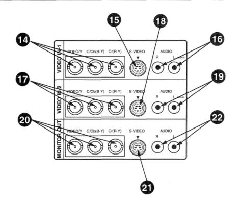
**14** Used to connect a video source to the projector.
