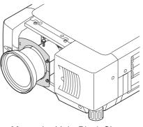
Mount the Light-Block Sheet with two (2) screws.
