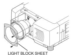
Make sure the sheet figure is correct and put in proper position.
