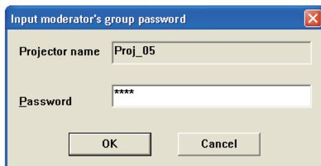
Enter a password and click **OK** button. When the password is authenticated correctly, the client can join in the moderator's group. The input password is registered in the moderator's password of the client.
