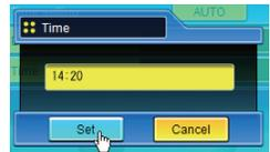
This projector does not provide the built-in battery. The date and time information are lost when the projector turns off ( when "Eco" is set for the stand-by mode (Refer to p.74)), or the network configuration is reset. The timer function is disable until time is set up correctly. When using the NTP address for time setting, the current time is acquired at the projector starting up and the timer function is activated after finishing the time setting correctly.
