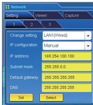
4. To apply the setting, press Set button. The network of the projector starts re-booting and applies the setting. It takes about 20 seconds to complete. Close the web browser and access to the login page again in 20 seconds.
