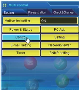
The multi controllable menus are "Power & Status", "PC adjustment", "Control", "Setting", "E-mail setting", "Timer", "SNMP setting" and "Network Viewer". Click each menu and perform setting and adjustment.
