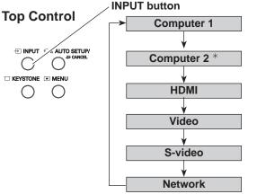
\* COMPUTER 2 can not be selected when using the COMPUTER IN 2/ MONITOR OUT terminal as MONITOR OUT output.
