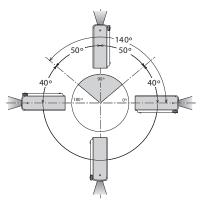
Be sure to set the Lamp control in High and the Fan control in On 3 in the setting menu when using the projector inclined at between +40 degrees to +140 degrees to the horizontal plane at altitudes between 0 and approximately 1,600 meters above sea level.
