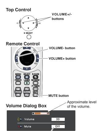
Press the MUTE button to set the Mute function **On** or **Off**. The dialog box disappears after 4 seconds.
