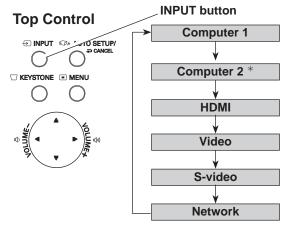
\* **COMPUTER 2** can not be selected when using the COMPUTER IN 2/MONITOR OUT terminal as MONITOR OUT output.
