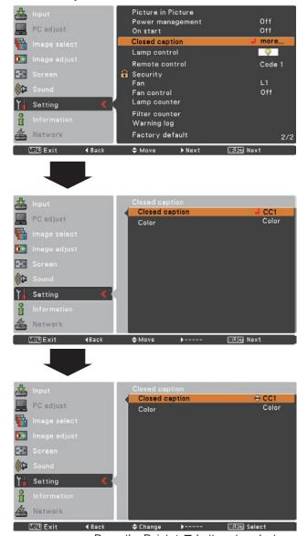
Press the Point ▲ ▼ buttons to select **Off, CC1, CC2, CC3** or **CC4**, and then Press the SELECT button.
