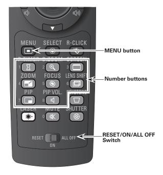
Press and hold the MENU and a number button (1–8) that corresponds to the remote control code for more than five seconds to switch between the codes.
