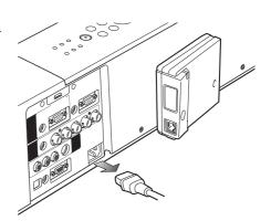
$\boldsymbol{3}$  Connect the UTP straight cable to the hub.
