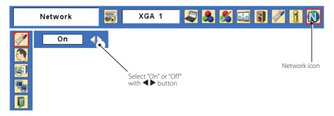
The network unit begins restarting each time the mode is set "On".
