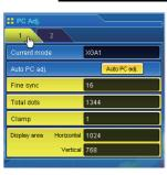
Current mode.....Displays a current mode like VGA, SVGA, XGA. SXGA, UXGA, WXGA, etc. or MODE1 - MODE10, EXT11 -EXT50 which are the customized mode created by using the "Mode Store" function described below. EXT51 - EXT60 represents mode Totalsave1 -Totalsave10 used in the item "Save" (☞p.56).
