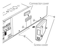
$oldsymbol{3}$  Tighten two screws by using a coin etc.
