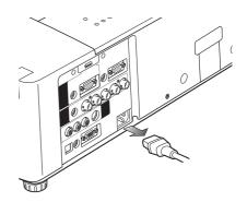
**2** Remove the connector cover and screw covers (2 pieces) from the projector and insert plug on this product to the option connector.
