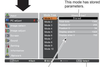
Values of **Total dots**, **Position H**, **Position V**, **Display area H** and **Display area V**. Press the SELECT button to clear the stored data.
