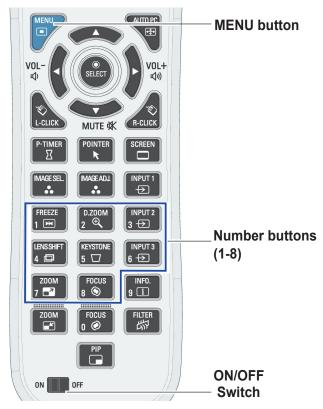
Press and hold the MENU and a number button (1-8) that corresponds to the remote control code for more than five seconds to switch between the codes.
