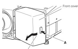
Pull this part forward with pushing button **A**.
