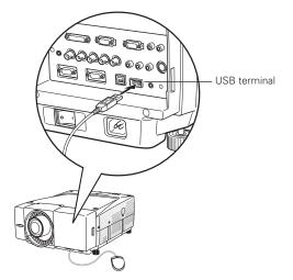
Connect the USB terminal on the projector and a USB mouse when operating the projector's menu with the USB mouse. A mouse cursor will appear on the screen with the mouse connected.
