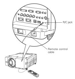
Connect the R/C JACK on the projector and the remote control with the remote control cable when operating the remote control as wired.
