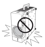
Do not place on an unflat surface and check no object under the cabinet.
