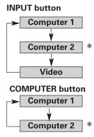
Computer 2 is not displayed when the COMPUTER IN 2/COMPONENT IN/MONITOR OUT terminal is used as Monitor out.
