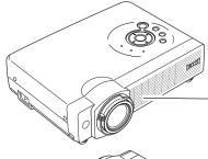
Openings in the cabinet are provided for ventilation and to ensure reliable operation of the product and to protect it from overheating, and these openings must not be blocked or covered.
