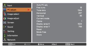
Use Point ▲ ▼ buttons to select **Auto PC adj.** and press the SELECT button. **Please wait...** appears while the Auto PC adjustment is in process.
