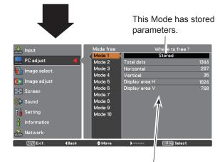
Values of **Total dots**, **Horizontal**, **Vertical**, **Display area H** and **Display area V**.
