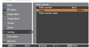
Press the SELECT button to select Timer, and then use the Point ▲ ▼ buttons to set the timer. Select from (Off/1000H/ 2000H/ 3000H/4000H/5000H/6000H) depending on the use environment.
