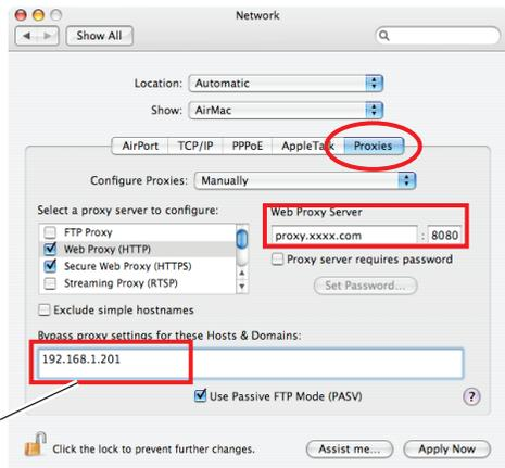
To designate proxy settings that will not use the proxy server when accessing the projector installed in the local area network, enter the IP address or domain name here.
