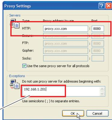
To designate proxy settings that will not use the proxy server when accessing the projector installed in the local area network, enter the IP address or domain name here.
