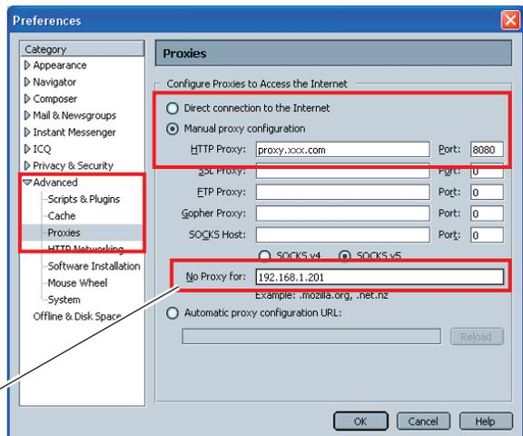
To designate proxy settings that will not use the proxy server when accessing the projector installed in the local area network, enter the IP address or domain name here.
