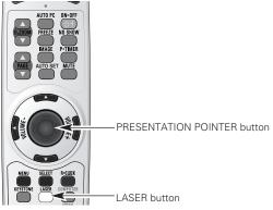
After the Laser pointer has switched to the Pointer, use the LASER button as the Pointer function ON-OFF switch. Press the LASER button toward the projector and see if it lights green.
