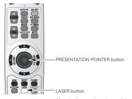
After the Laser pointer has switched to the Pointer, use the LASER button as the Pointer function ON-OFF switch. Press the LASER button toward the projector and see if it emits green light.
