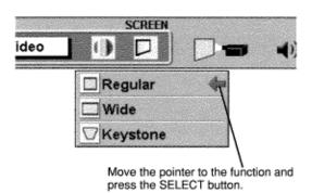
NOTE:The Regular and the Wide cannot be operated when "720p," "1035i," "1080i-50" or "1080i-60" is selected on SYSTEM MENU (P33).
