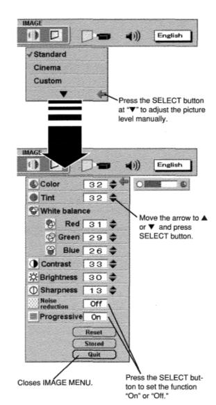
NOTE: The Noise Reduction cannot be operated when the video signal is from the Y, Pb/Cb, Pr/Cr jacks.
