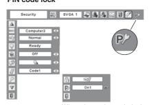
When the projector is locked with the PIN code, the PIN code lock mark appears on the menu bar.
