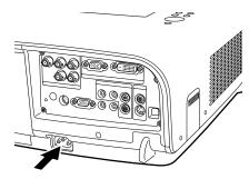
Connect the AC power cord (supplied) to the projector. The AC outlet must be near this equipment
