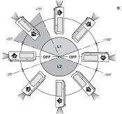
\* When installing the projector in upwawrdly inclined position, install the projector bottm side up.
