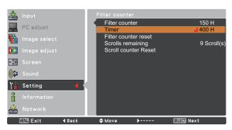
Press the SELECT button to select **Timer** and then use the Point ▲ ▼ buttons to set the timer. Select from (**Off/400H/700H/1000H**) depending on the use environment.
