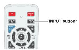
\* Only the Input button function is set Mode 1 in the Setting menu, the INPUT button is used for switching input source.
