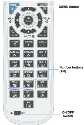
Press and hold the MENU and a number button (1-8) that corresponds to the remote control code for more than five seconds to switch between the codes.
