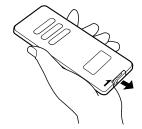
Replace with new battery. Install with battery (+),(-) marks properly.
