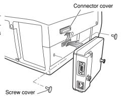
**3** Tighten two screws by using a coin etc.
