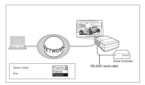
Please use a serial cable supplied with your projector or a commercial serial cable which has ferrite cores at the both cable ends.
