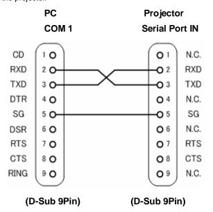
Connect COM port of the computer to SERIAL PORT IN of the projector.
