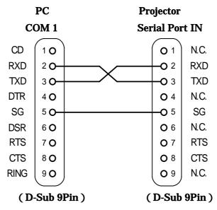
Connect COM port of computer to SERIAL PORT IN of COM Port.
