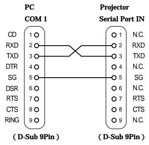
Connect COM port of computer to SERIAL PORT IN of COM Port.
