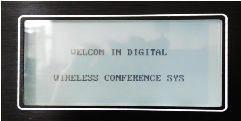
The welcome screen will be displayed about 5 seconds; the system automatically enters the standby.
