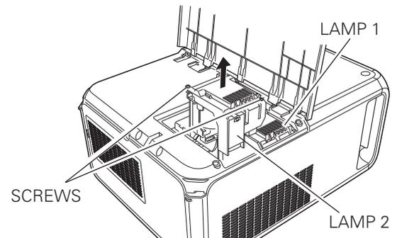
Make sure which number of lamp needs to be replaced on Lamp Status Display. Figure shows case of replacing LAMP 2.
