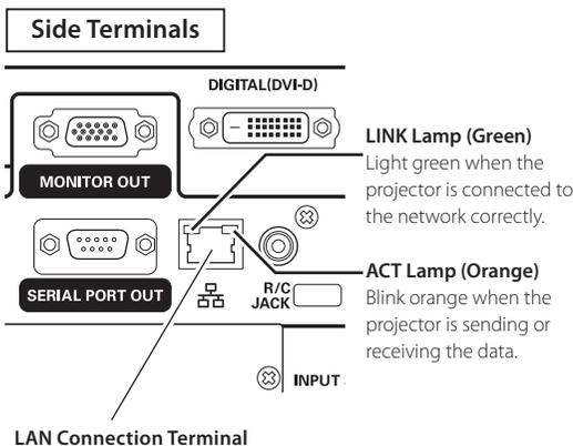
3. Select "Network setting" in the Network menu with the Point ▲▼ buttons and press **SELECT** button, and then the LAN setting screen will appear and selected LAN settings will be displayed. Adjust each item to the setting environment. Consult your system administrator about the detailed settings.
