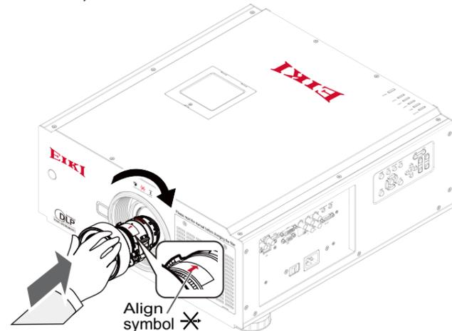
3. Make sure the lens is pushed into the holder and turn it clockwise to the "Lock" position. When turning the lens, the "Click" sounds once to indicate that the lens is completely fixed.
