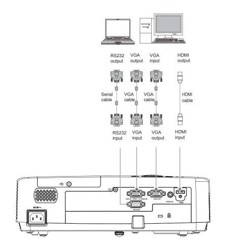
Unplug the power cords of both the projector and external equipment from the AC outlet before connecting the cables.
