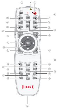
\* Laser Transmitting Window: Laser beam will emit from this window while pressing LASER button during the projection to use the remote controller as a laser pointer.
