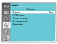
Store....The keystone correction will be kept when plug out the power cord or turn off the projector.
