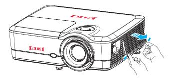
**4.** Slightly move the dust filter cover to the left and to the right direction to release it from the latches on the case. And then remove.
