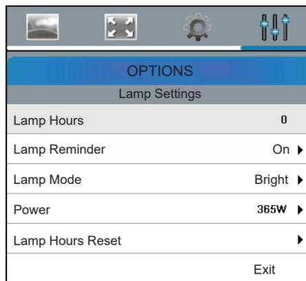
4. Use the arrow keys (▲▼) to select **Lamp Hours Reset** and press the **Enter** button to enter its submenu.
