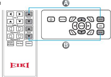
**3.** Use the **Keystone H** buttons (on the remote control) to adjust the keystone horizontally and make a squarer image. Use the **Keystone V** buttons (on the remote control) to adjust keystone vertically and make a squarer image.
