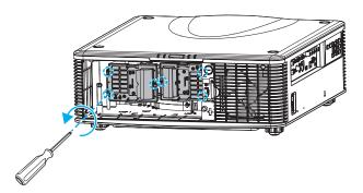
**5.** Carefully remove the lamp module(s).
