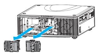
${f 6.}$  Install the new lamp module(s) by reversing the previous steps.
