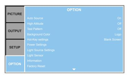
**3.** Use the arrow keys (▲▼) to select **Light Source Settings** and press the **Enter** button to enter its submenu.
