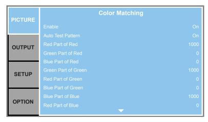
You may require a unique color gamut (range) for a single projector or application, or you may need to precisely match colors across multiple adjacent displays. Use Color Matching by Meter Adjustment or by Manual Adjustment to define the precise hue of each primary color component (red, green, blue and white).
