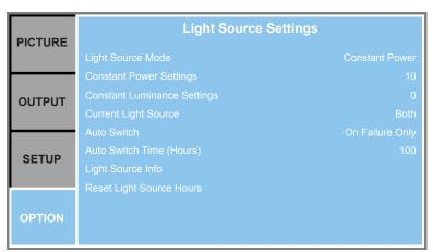
**4.** Use the arrow keys (▲▼) to select **Reset Light Source Hours** and press the **Enter** button to enter its submenu.
