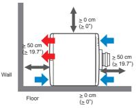
Caution-When installing the projector on the left side, leave a space of at least 50 cm between the exhaust vent and the wall and a space of at least 50 cm for the intake vent.
