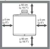
Caution-When installing the projector on the right side, leave a space of at least 50 cm between the exhaust vent and the wall and a space of at least 50 cm for the intake vent.
