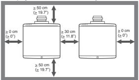
■ Caution- For 360° installation, install the projector more than 50 cm away from the wall or the floor. When the air intake and discharge outlet are obstructed, the temperature inside the projector will rise and this may result in a malfunction.
