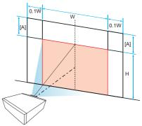
[A] differs when different lens is installed.
