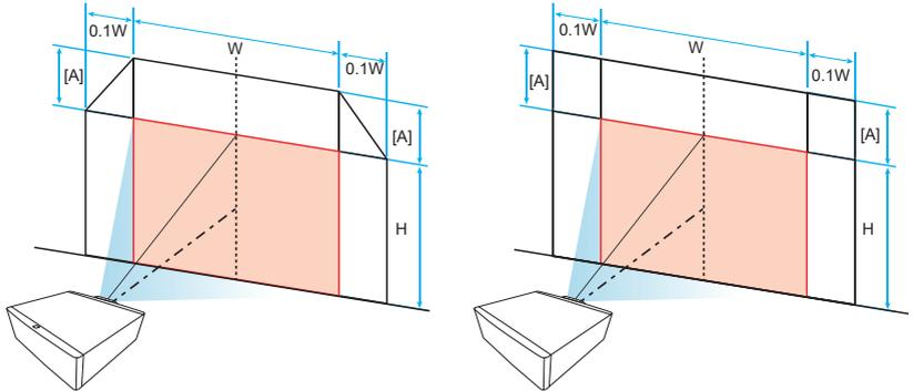
[A] differs when different lens is installed.
