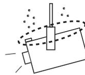
When hanging the projector from the ceiling, clean the air intake vents and top of the projector periodically with a vacuum cleaner. If you leave the projector unclean for a long time, the cooling fans can be clogged with dust, and it may cause a breakdown or a disaster.
